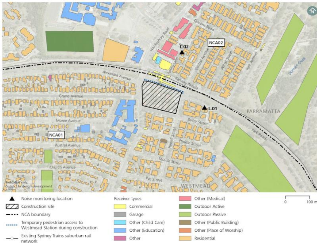
Figure 16 Location of sensitive receivers near Westmead site
