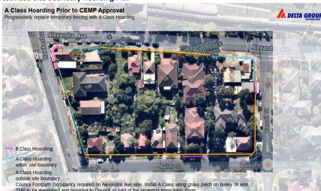
Figure 4 Westmead Site Boundary Hoarding Plan
