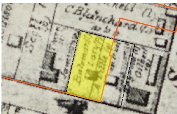
Figure 4.7 Detail from Brownrigg's 1844 survey showing a masonry building (as it is shaded) in Lot 74. (Source: SLNSW with GML overlay)
