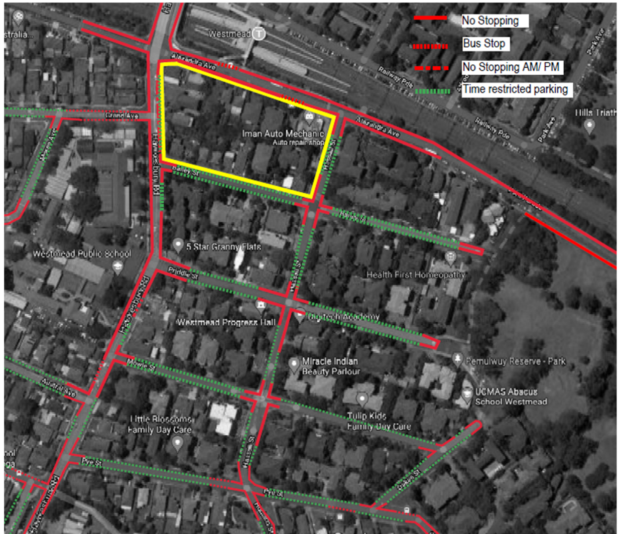
Figure 7: Existing parking restrictions
