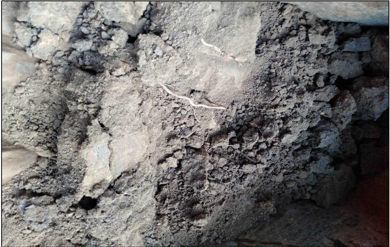
**Photograph 15:** Close-up of view of typical fill materials observed throughout site, observed at test pit 2.
