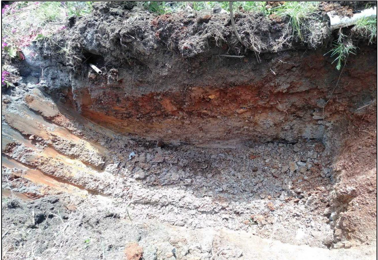
**Photograph 13:** Representative fill and natural materials at test pit 9. Date: 15.11.21.
