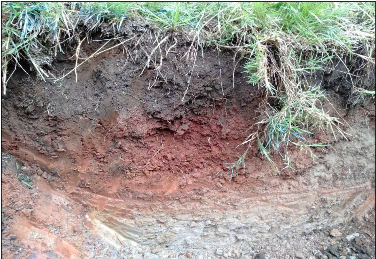
**Photograph 12:** representative fill and natural materials at test pit 12. Date 23.11.21.
