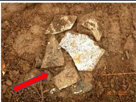
**Photo 11:** Ground surface north of 33 Bailey Street following rainfall event – debris from previous photo uncovered to confirm asbestos.
