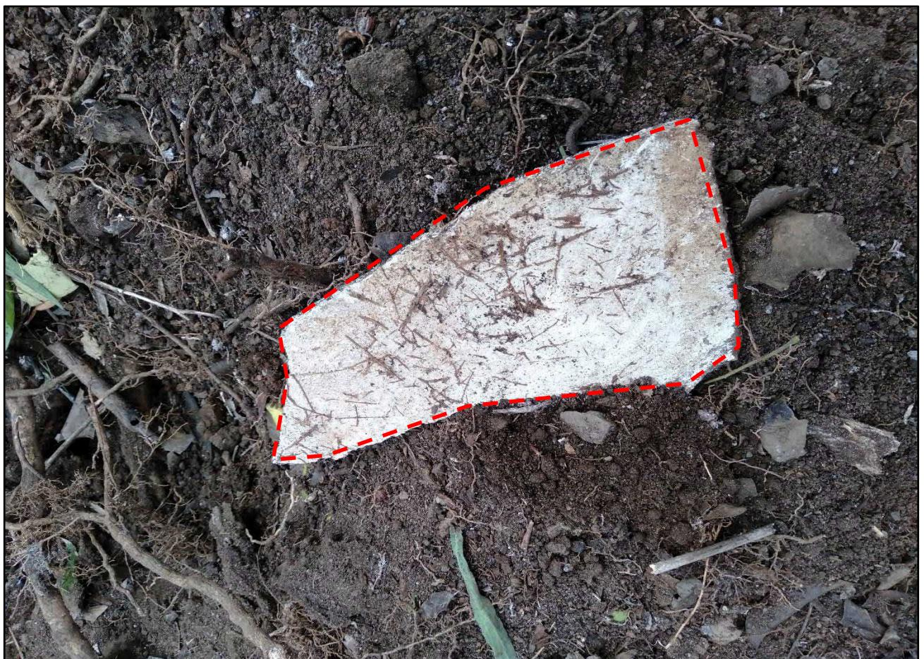
**Photograph 8:** Representative asbestos sheeting, observed at TP10, within the registered asbestos area. Date: 15.11.21.
