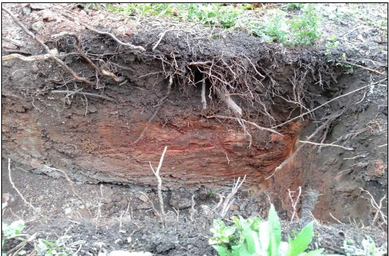
**Photograph 10:** Representative fill and natural materials, observed at test pit 20. Date: 24.11.21.
