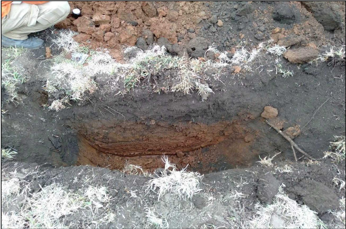
**Photograph 11:** Representative fill and natural materials, observed at test pit 5. Date: 24.11.21.
