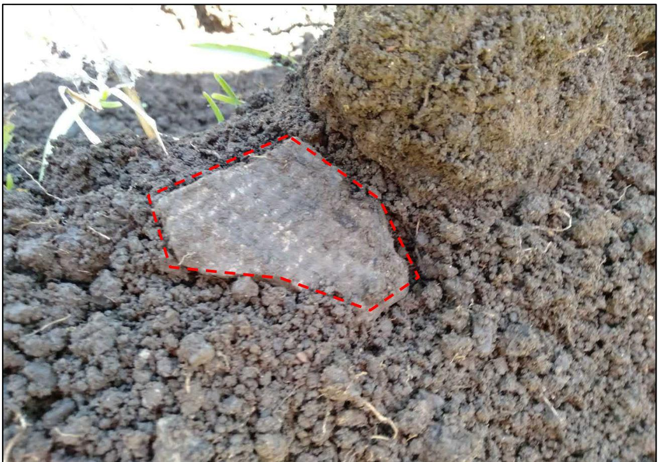
**Photograph 6:** Representative asbestos fragment, observed at TP2. Date 12.11.21.
