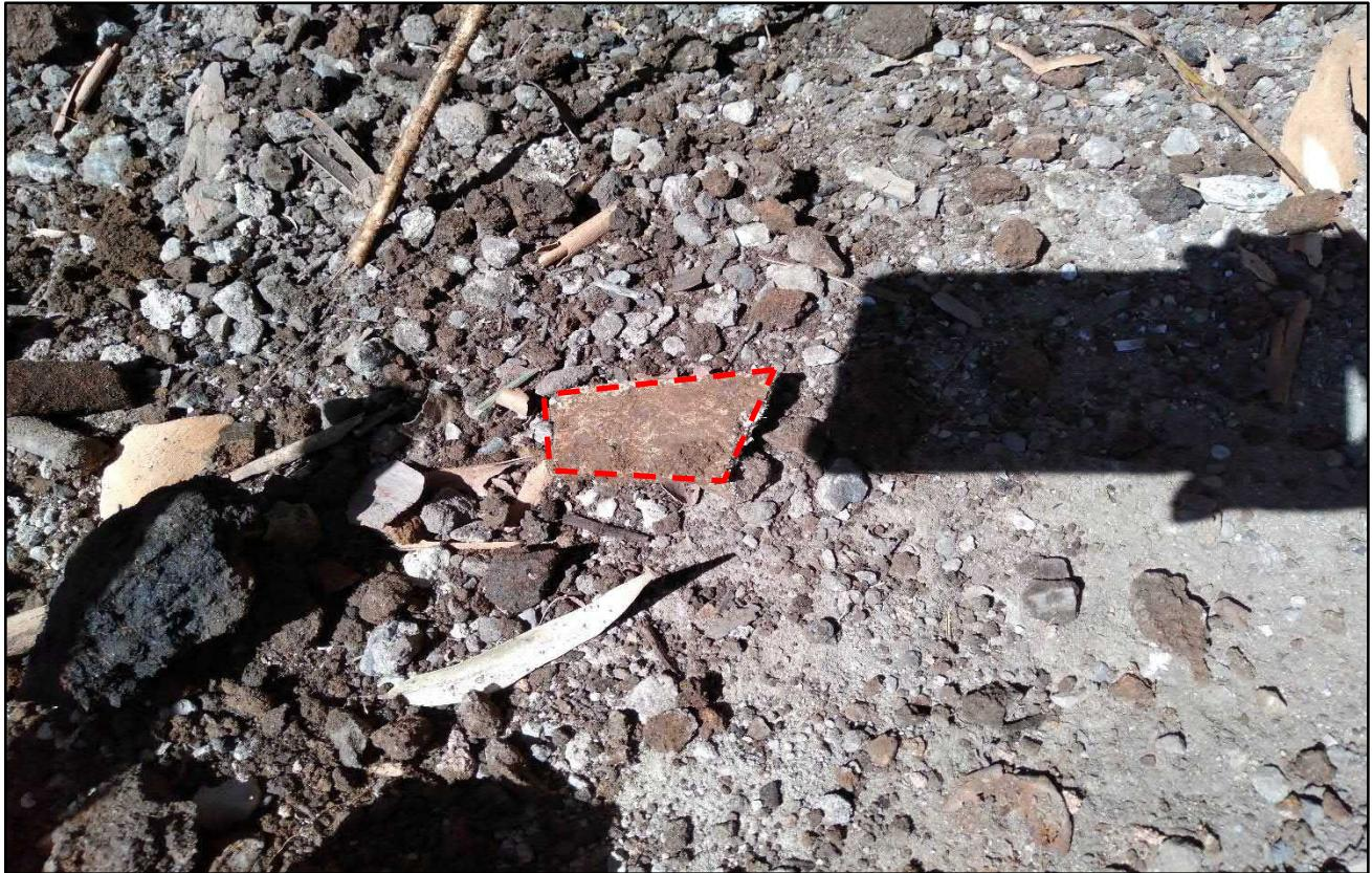
**Photograph 7:** Representative asbestos fragment, observed at test pit 3. Date: 15.11.21.
